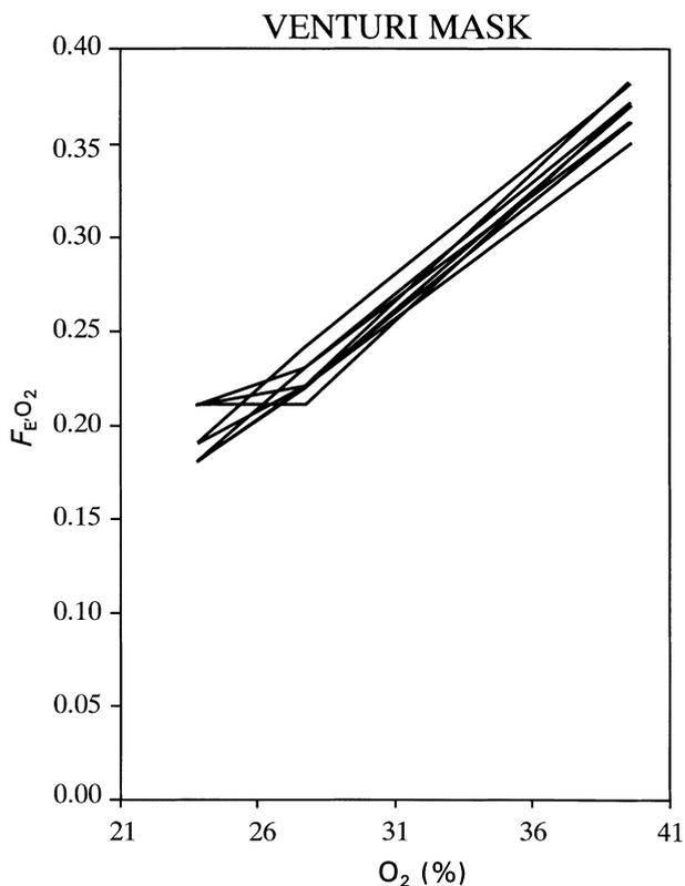
**Figure 3** Expired oxygen fraction plotted against set oxygen percentage for the Venturi masks.
